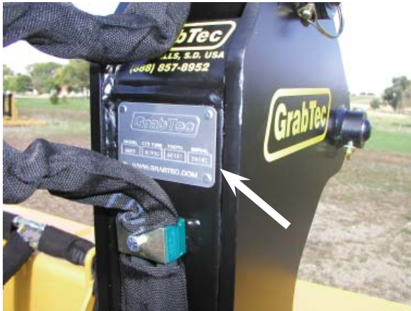
The Serial plate is typically found on the rear of the right side torque tube.
